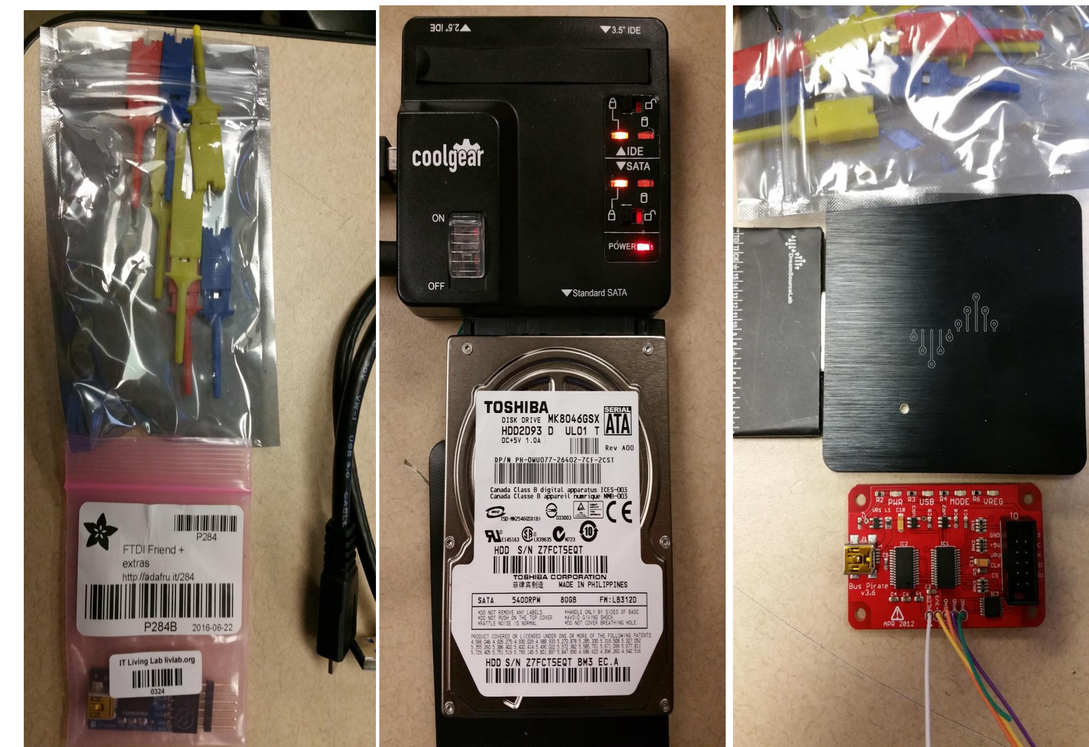
Tools provided(left to right CW): Connection pins, FTDI Friend , write-blocker, Logic Analyzer, Digital Microscope, USB HD Docking Station “Toaster” and DS-View software
